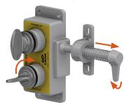
By inserting and turning the isolation key in the AIE, the personnel key can be turned and released. This traps the isolation key, which enables the release of the side bolt. The personnel key should be returned by the operator while in the hazardous area. Isolation key is trapped, the side bolt and personnel key are free.
