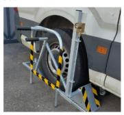
If the Double Chock K/KL is correctly installed, it loosely grips the wheel to be secured. Pull the locking lever upwards, the wedge moves together and must grip the wheel as tightly as possible.
