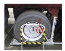
The Double Chock K/KL is correctly locked, the key can now be turned anti-clockwise and removed. When the key is turned, the Chock is locked in its setting.
