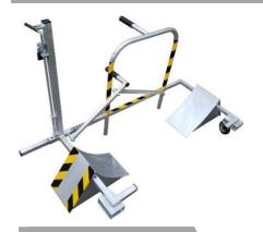
The Double Chock K/KL is a wheel chock that prevents vans, trucks and trailers from moving during loading and unloading. In combination with the Salvo system, the gate or doc leveller is interlocked with the Chock. This ensures safeguard against accidental drive aways. Like all existing products in the Salvo range, the Double Chock K/KL is based on Castell's proven key transfer interlocking.
