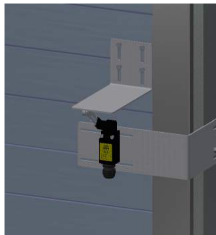
Special brackets required to fit to Pre-cast Concrete Installation
