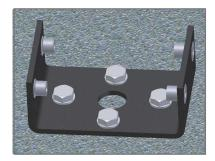
3 Lower the Bollard into place over the footplate.
