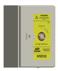
The KSD is a key driven non-fused switch disconnector suitable for power isolation. The standard KSD comes with either 4 or 6 poles plus 2 auxiliary early break contacts. The KSD is manufactured from either brass or stainless steel. It can be supplied either suitable for mounting into an existing panel, or in its own IP65 rated lockable mild steel enclosure.
